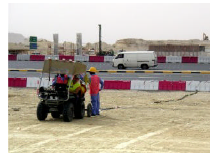
System for land survey of large areas. Note the geophone string (landstreamer) behind the quad bike.
